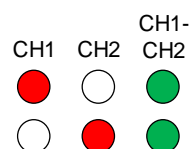
Figure 3-2: Channel selector indicator states.
