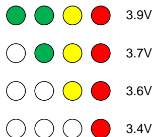
Figure 3-1: Battery voltage indicator states and corresponding voltages.
